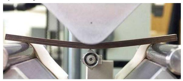
Fig. 7 Detail of three-point-bending device with sample.
