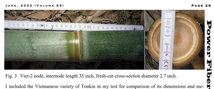
Fig. 3 Viet-2 node, internode length 35 inch, fresh-cut cross-section diameter 2.7 inch.
