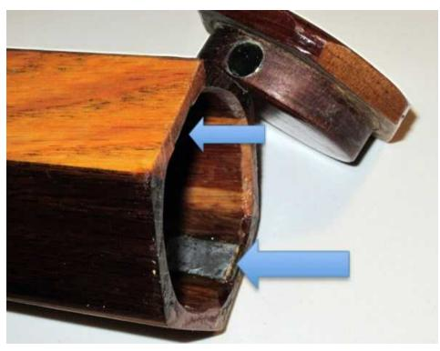
Figure 5 (Arrows denote small iron plate replacing inner magnet.)
