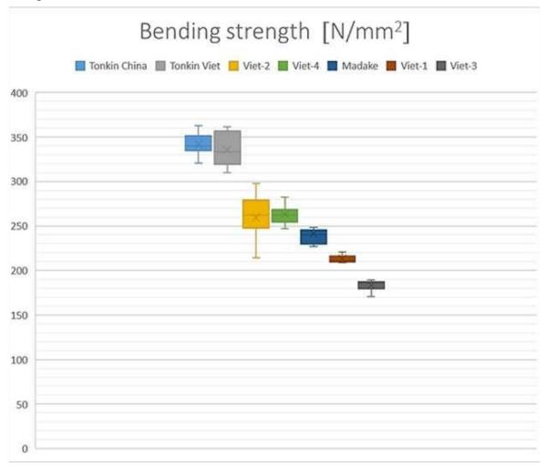
Fig. 8 Bending strength of the outer 3 mm (0.118 in) of seven bamboo species. Whisker-Boxplots showing mean, median, minimum and maximum values.
