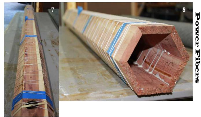
Once the glue has cured, I unwind the wrapping and take off any tape that's left from the process (see Photo 9).
