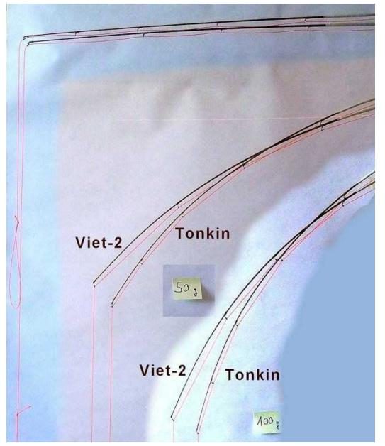
Fig. 20 Bending chart of a rod made from Tonkin and one from Viet-2 with same taper and length without weight and with 1.76, respectively 3.53 oz. attached to the tip.
