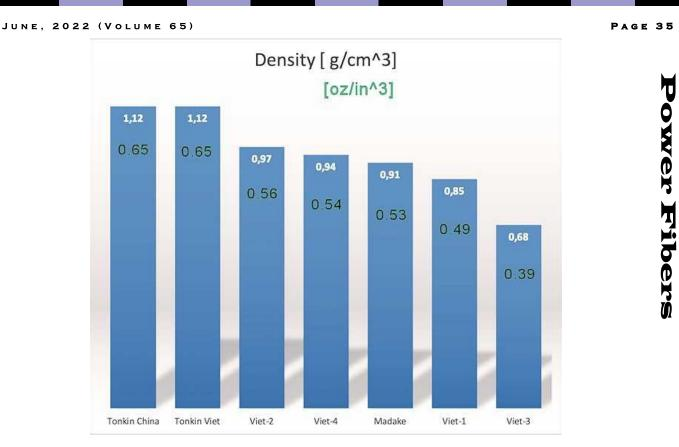
Fig. 10 Density of conditioned samples from the outer 3 mm (0.118 in) of seven bamboo species.
