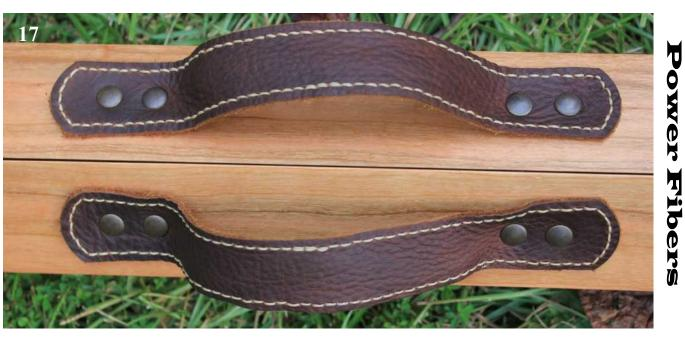
Next, I take care of the leatherwork. I cut my leather pieces for each build and hand stitch them all. I will cut two for each box. They're laid in place and installed using Chicago screws and some adhesive to make sure that they stay put (see Photos 17 and 18).
