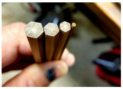
A few final points on building a splice rod, I did swell my joints 10% of the rod diameter at the center of the splice and continued the swell for the entire length of the splice. Also, it is important not to make the tip of your splice less than .040. As I stated earlier, I did hollow three sections of this rod and I made sure to stay 3.5" away from each of the splices.
