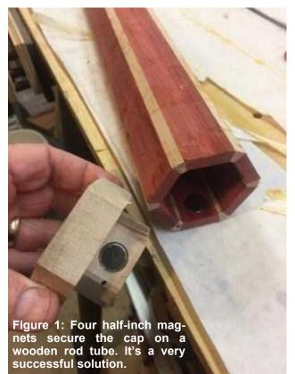
(Figure 1). It's easy to implement and very secure. The basket-weave tube, however, has a rounded cap (Figure 2). This necessitated using a smaller magnet. In hindsight, I should have doubled the number of magnets. At the show, I dropped the tube and the cap popped off and rolled under a table. My next tube needs a better solution. Obviously, I could use a leather strap and buckle like so many craftsmen use, but that's just never been appealing to me. We all have our quirks.
