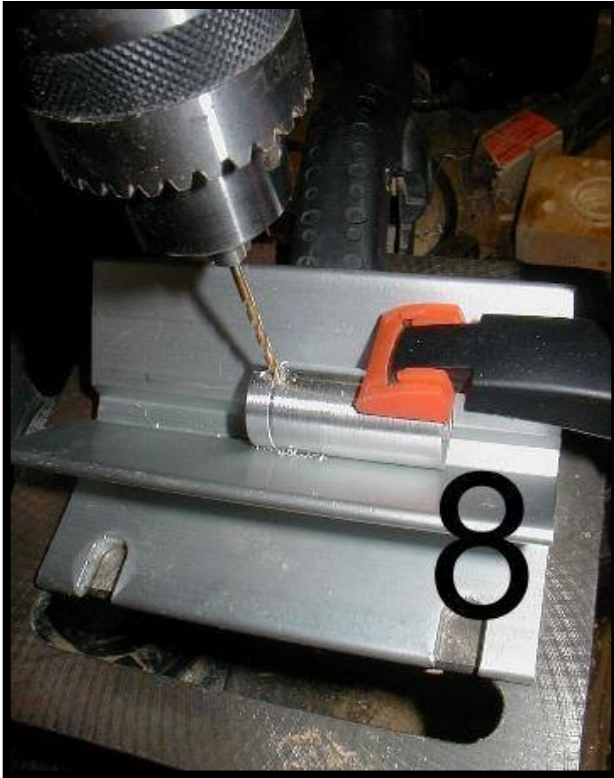
Drill holes for the screws. Use a #29 drill bit to create a hold to tap an 8/32 thread (Photo 8).
