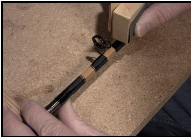
Sanding the thread wraps after the fifth coat of finish.
