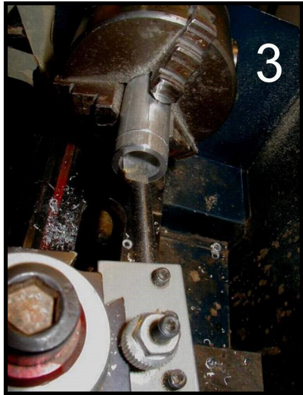
Now we need to remove the inner burr with a boring bar (Photo 3).
