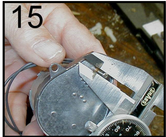
Measuring OD of motor shaft (Photo 15).
