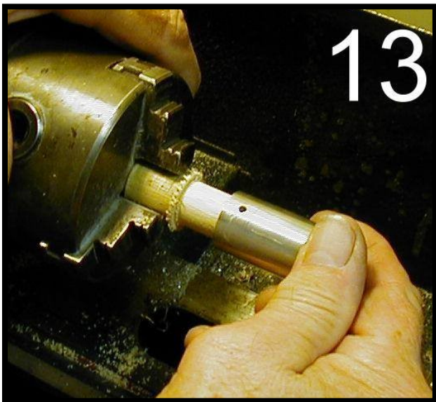
Check the fit of the plug to the body of the chuck often for a snug fit (Photo 13).
