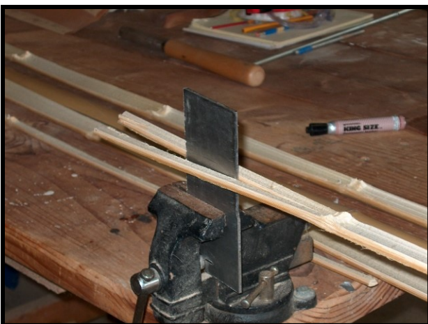
Splitting into narrow strips.
