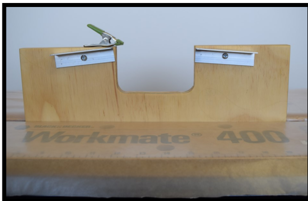
Clamp both sections into the jig and adjust as needed. I use Gorilla Glue for my scarf joints. Lightly moisten the strips, and then apply a thin layer of glue to each joint surface. Wrap each joint tightly with the same binding thread you use on rod sections. Remove the joined sections from the jig and make any necessary
