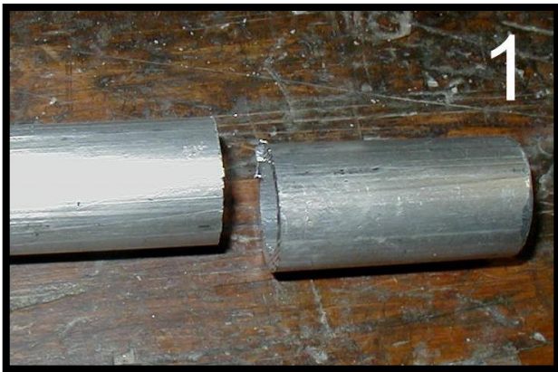
First, I cut a three inch length of thick wall aluminum pipe (Photo 1).
