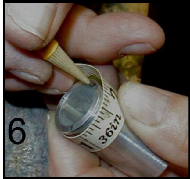
Place three equal marks around the tube. These will show the location for three screw holes (Photo 6)
