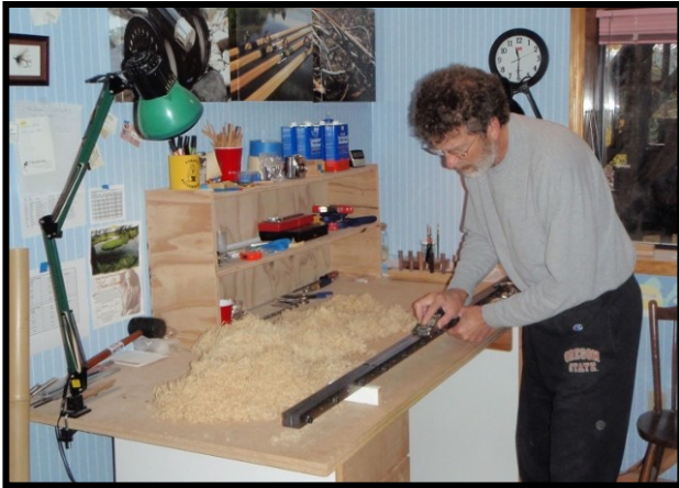
Hand Planing gets the strips down to the final tapered dimensions.
