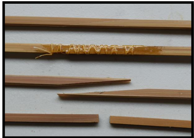
Almost all bamboo strips will have a slight 'sweep' curving away from the power fiber surface. My binding jig is adjustable for this 'sweep' and allows the actual joint area to be aligned accurately.
