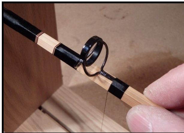
Wrapping a Black Banded Agate Stripping Guide.
