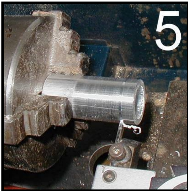
Using a parting bit, cut a groove a half inch from the front end (Photo 5). This will be the line to drill and tap the screw holes
