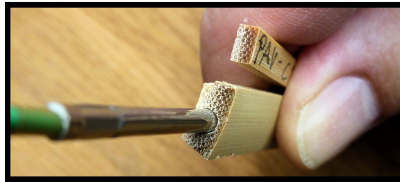
Fig. 14 Temperature sensor inside Tonkin. The upper sample is 3 millimeters (0.118”) thick.
