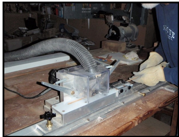
After heat treating, the bamboo strips are roughed out into a triangular shape on a Bellinger Beveler.
