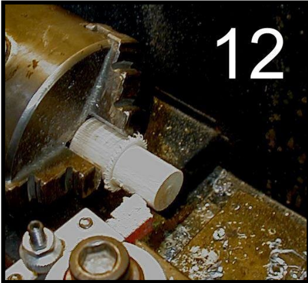
I decided to turn a length of dowel to fit the ID of the chuck body. This dowel should be a snug fit about 3/4 inch long (Photo 12).
