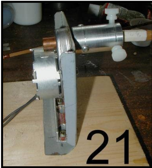
Photos 21, 22 and 23 show the rod ends inserted in the chuck.
