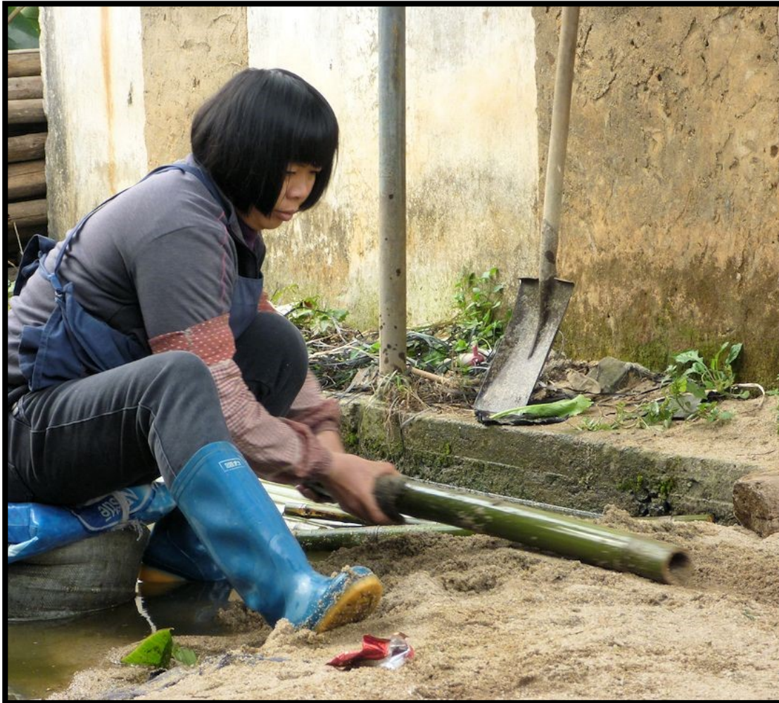
Fig. 10 Removal of the natural wax layer with sand and water.
