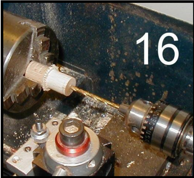
Drill a center hole for the motor shaft. This hole needs to be a really snug fit on the motor shaft (Photo 16).
